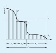
Fig. 11.2 Relations between bearing load and rotation speed
