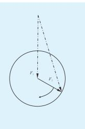
Fig. 11.4 bearing load composed of F1 and F2.
